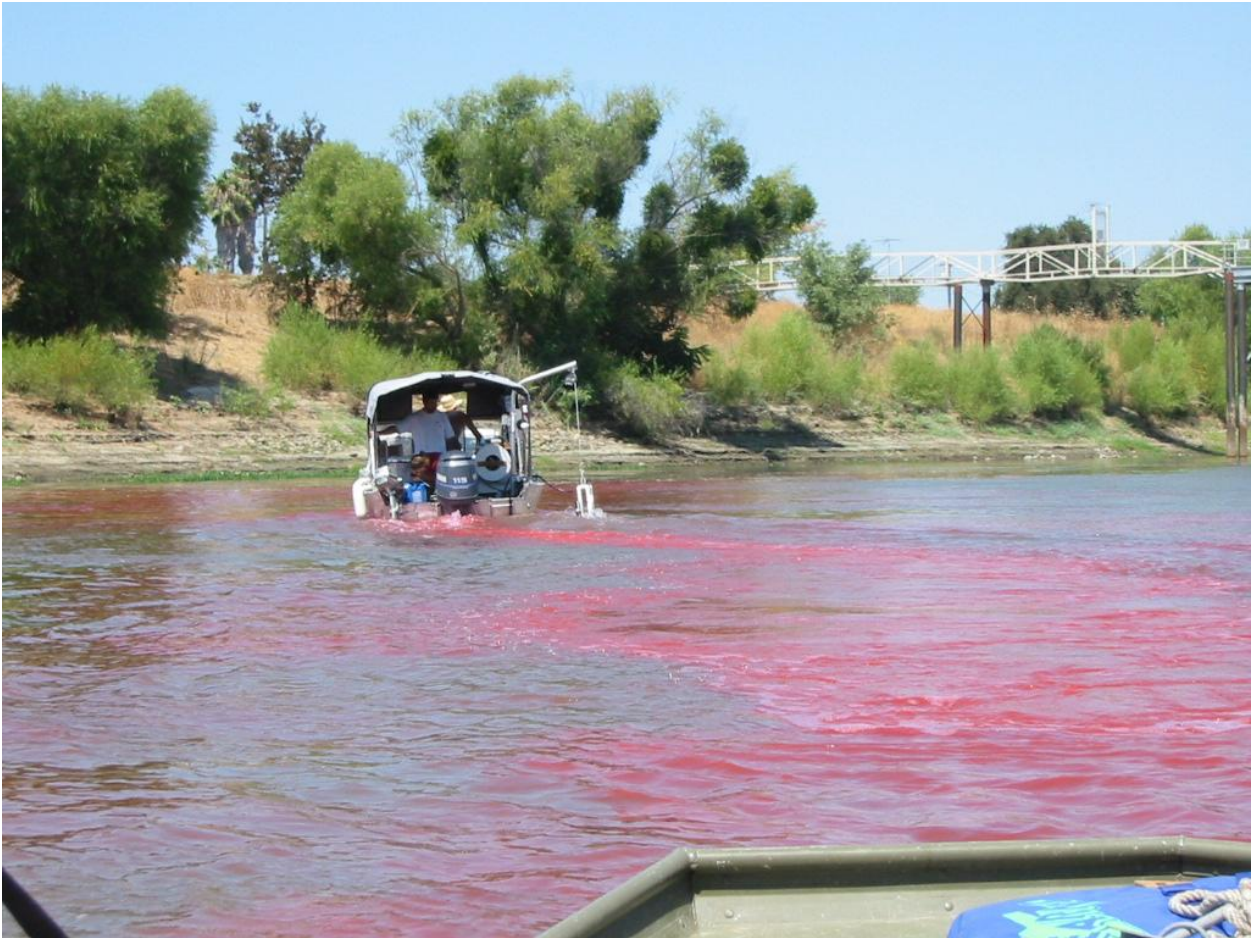
Figure 8. Rhodamine WT dye dispersal from Litton research vessel with Jon boat riding in the wake of the larger boat to assist with vertical mixing of the dye. Uniform mixing within the water column was achieved within 2 – 3 miles downstream. The research vessel then drifted downstream attempting to stay with the dye concentration peak.
