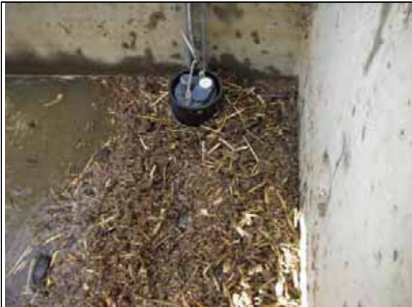
DO-130 Marshall Rd Res Entrance Sonde had a lot of debris in housing. The housing was lowered to prevent debris accumulation.
