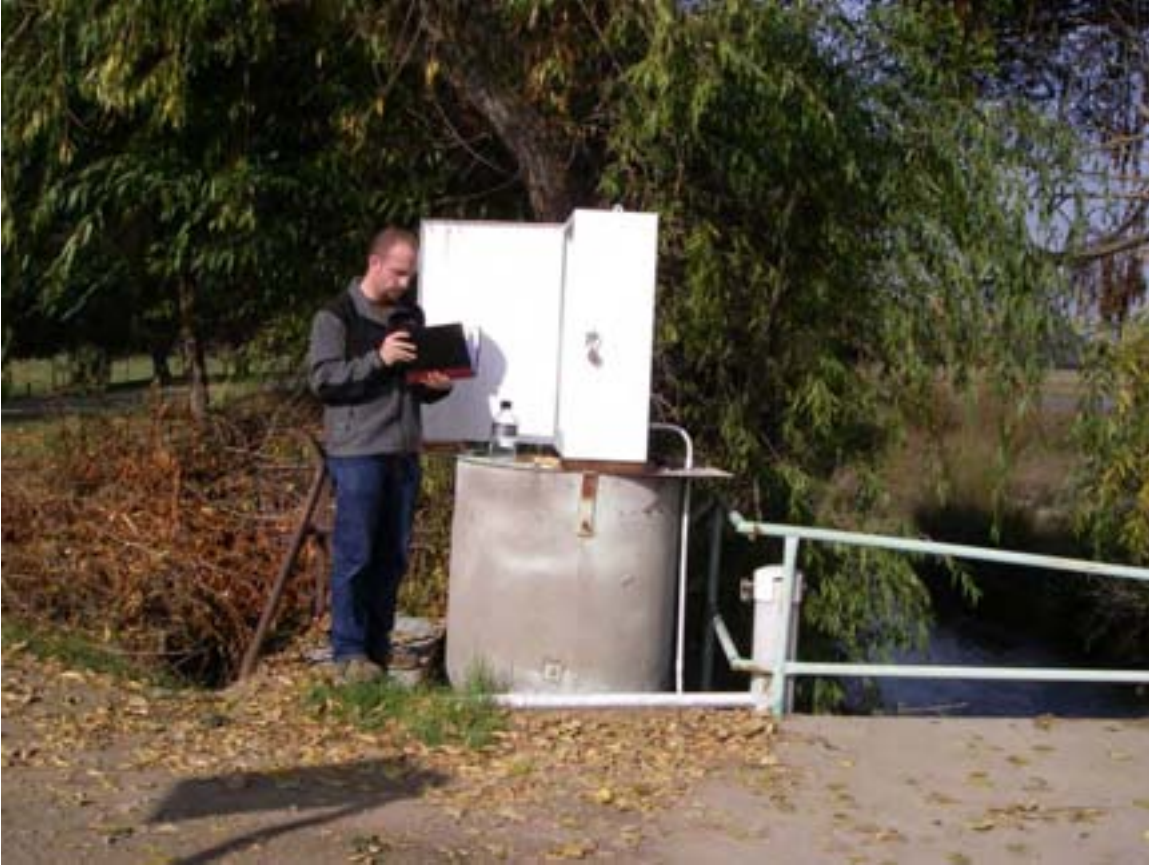
Figure 22: A Design Analysis Smartgas system was added to the Stevens chart recorder in late 2007, providing higher quality data.
