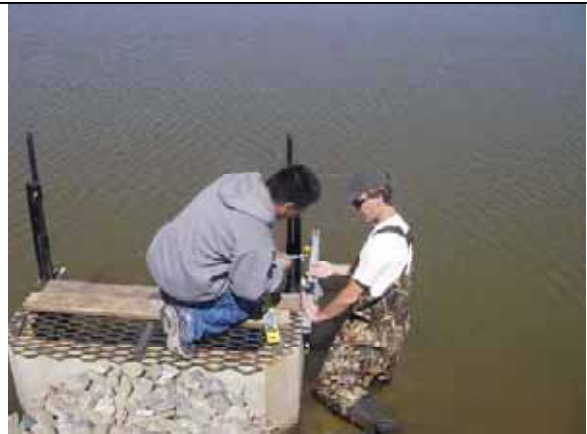
DO-132 Marshall Rd Res Pond 1 West Jeremy Hanlon and Student Intern mount the sonde to the side of the weir box.
