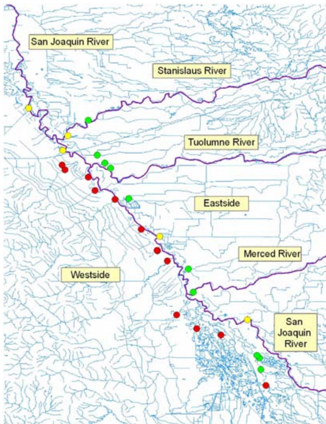
Fig. 4. Geographical analysis of turbidity (NTU) in tributaries of the San Joaquin River using normalized rank mean (NRM) analysis. Sites displayed in red have higher turbidity compared to the other tributaries combined (90% probability). Sites in green are significantly better than the mean for turbidity. Yellow locations are not different from the mean.
