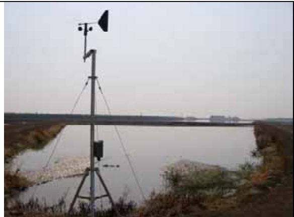
DO-130 Marshal Road Res Inlet Picture of the weather station at Marshall Road Reservoir. The station collects wind, air temperature and barometric pressure data.
