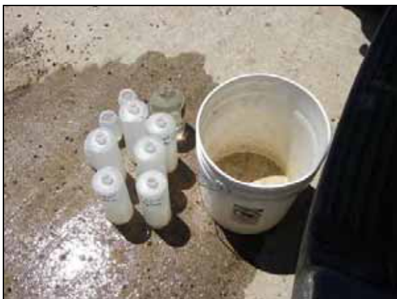
DO-29 TID Harding Drain Sample bottles set up for bucket sampling.
