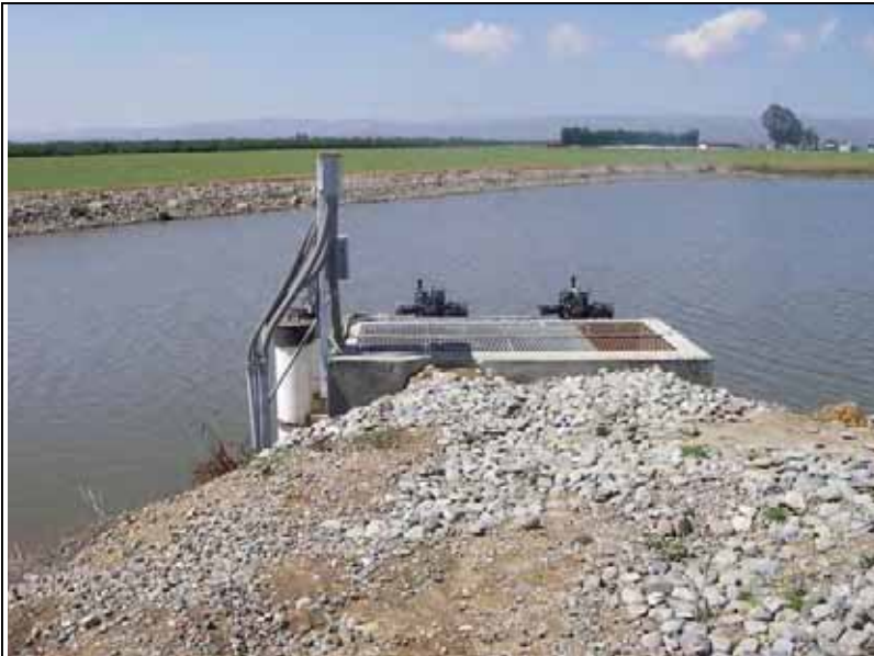
DO-131 Marshall Rd Res Exit Sonde was deployed off the side of the exit structure. The sonde was in a plastic housing attached to the structure with a cable and padlock.
